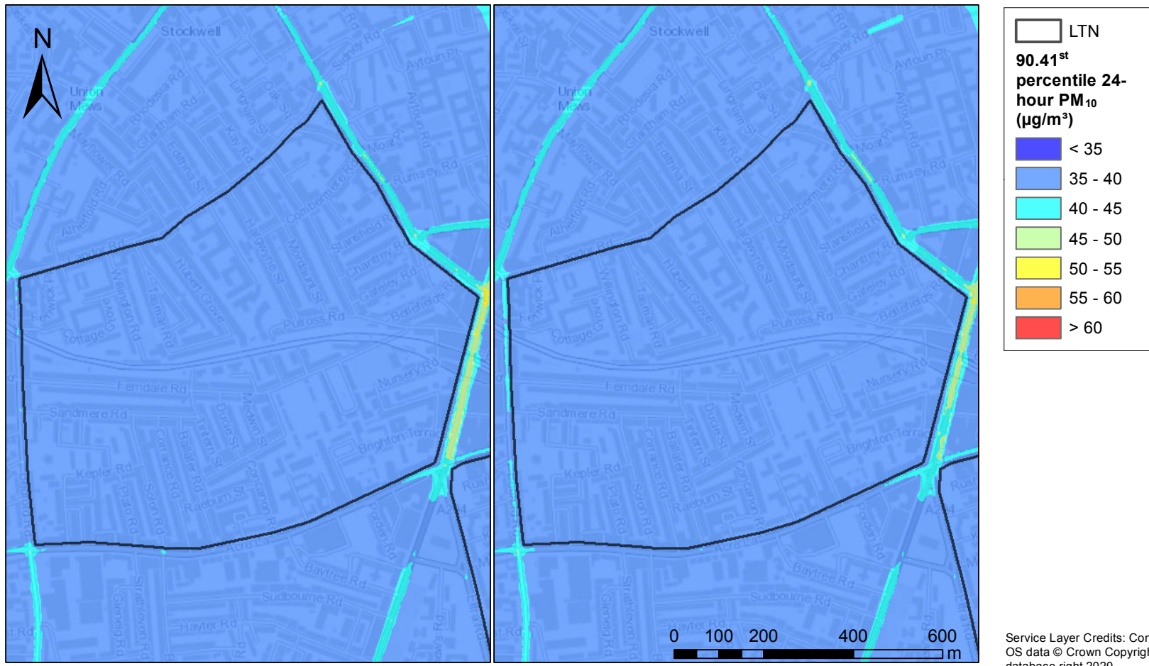
Figure 6.5: Pre-Scheme (left) and Post-Scheme (right) 90.41 st percentile of 24-hour average PM 10 concentrations (μg/m 3 ), Ferndale LTN
