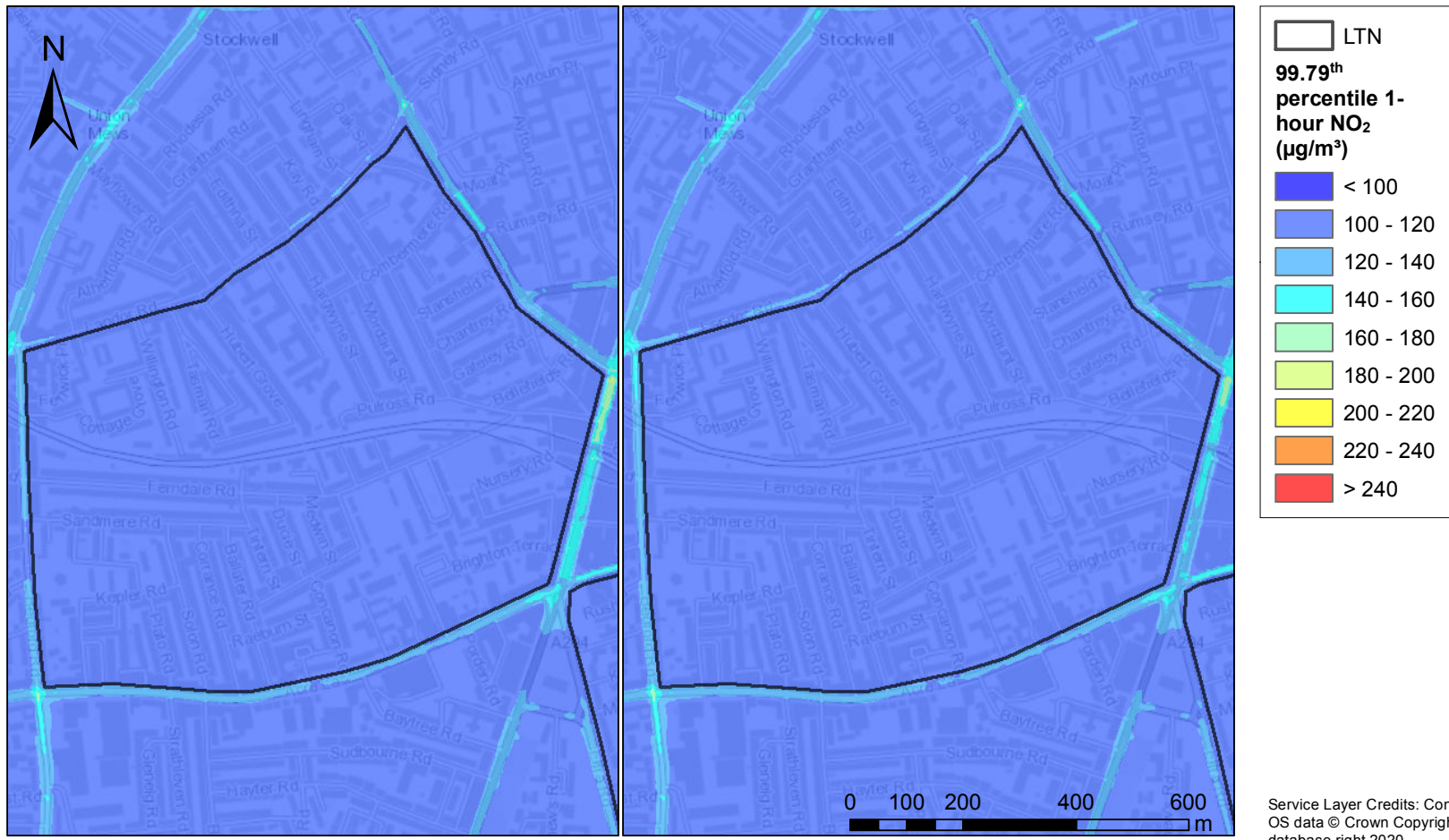
Figure 6.3: Pre-Scheme (left) and Post-Scheme (right) 99.79 th percentile of hourly average NO 2 concentrations (μg/m 3 ), Ferndale LTN
