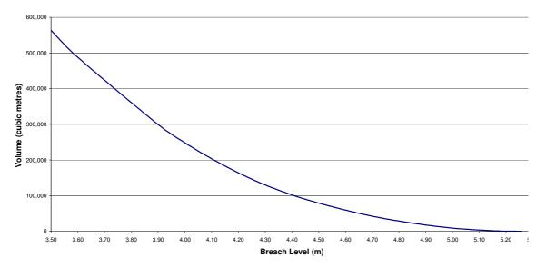
FIGURE C 4: MAXIMUM BREACH VOLUME FOR EACH ASSUMED BREACH LEVEL
