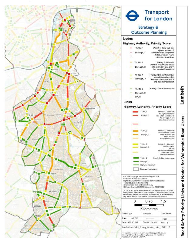
Figure 7: Priority links for collision reduction schemes
