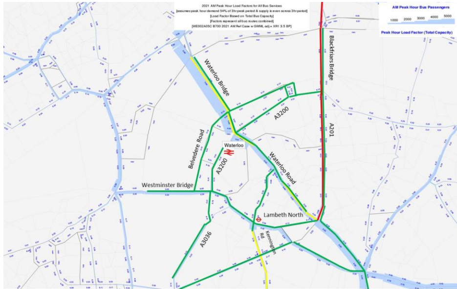
Figure 4.8: Bus Capacity Analysis: Waterloo (2021)
