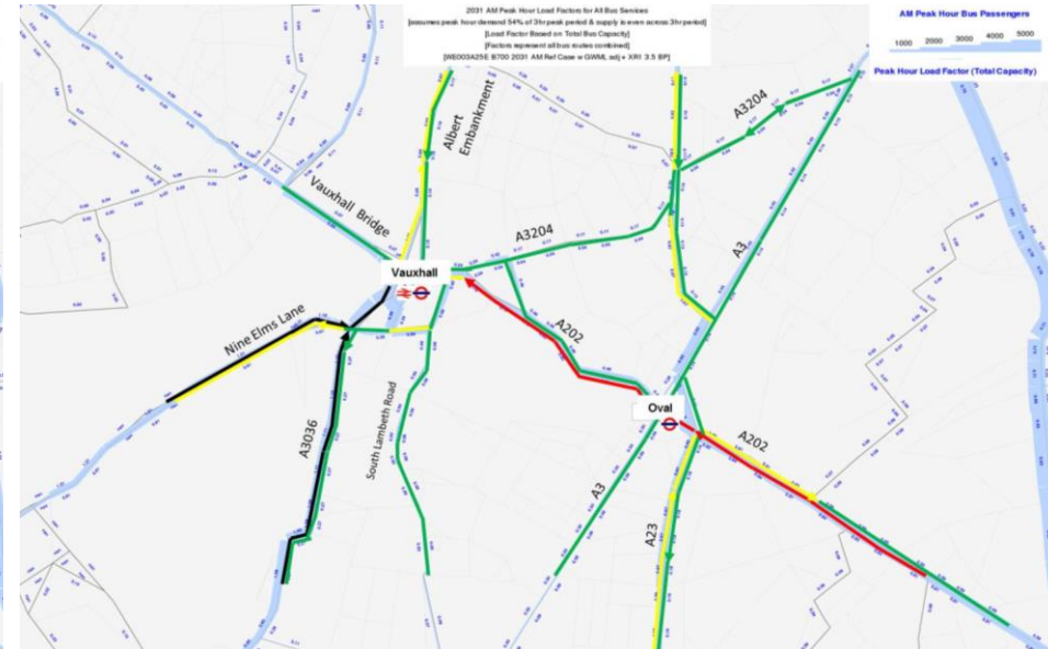
Figure 4.11: Bus Capacity Analysis: Vauxhall/Oval (2031)
