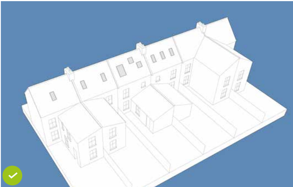
Figure 8: Rear roof lights at property nos. 1, 2 and 4 are considered appropriate as a general rule. On heritage assets noticeably smaller roof lights than those illustrated will normally be sought .
