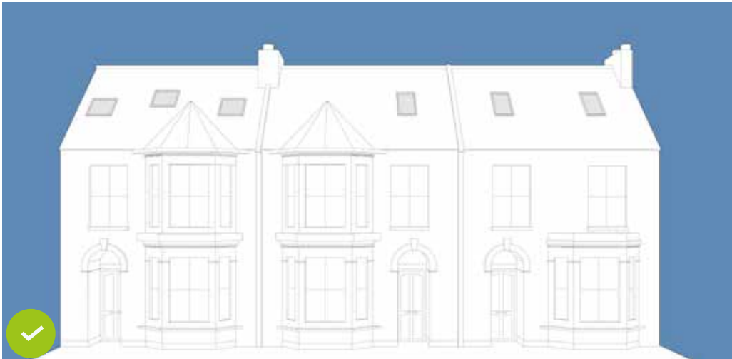
Figure 8: Front roof lights
