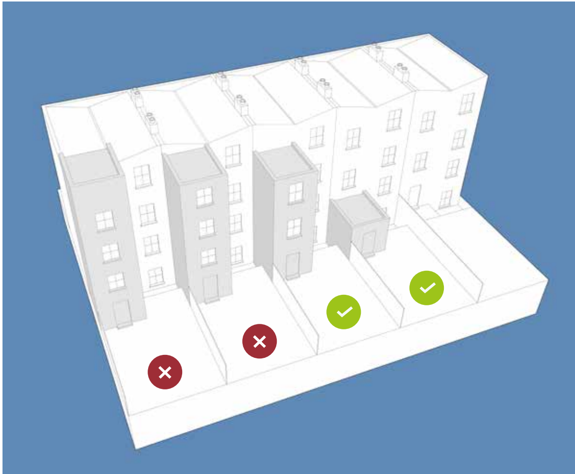
Figure 3: closet return extensions
