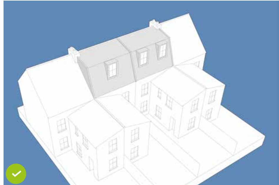
Figure 16: Traditional mansards (rear view)
